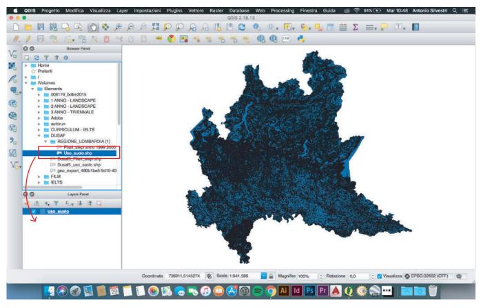
Step 1: Opening of the layer, drag the ".shp" file into the layers panel.
