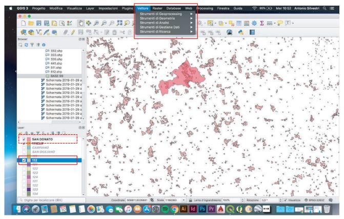
Step 13: "Clipping" of the layer inside the interested area. Open the inderested layers and click on "Vettore".
